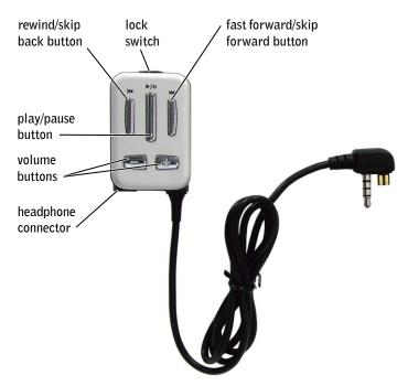
**REWIND/SKIP BACK BUTTON** —Press the rewind/skip back button to move to the start of the current track, or to go to the previous track. Press and hold the rewind/skip back button to move back within a track.
